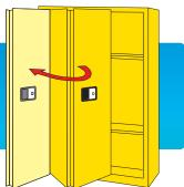
Bi-folding, Self-closing and Self-latching Door, with fusible link
