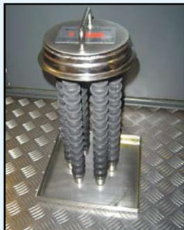
The core of the FILTRAMAG consists of six neodymium 'rare earth' magnetic rods offering an incredible 11,000 Gauss magnetic performance.
